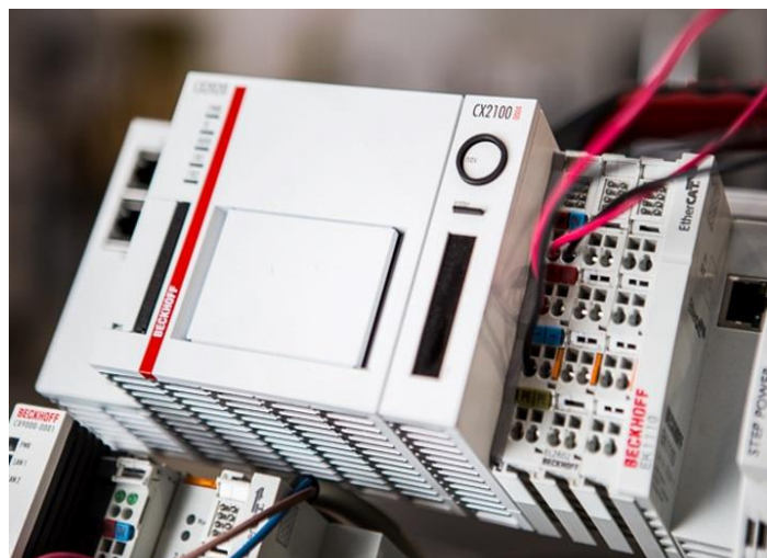
Figure 3.1.1: A typical PLC with one slot 16 inputs and 2 slots of 16 outputs
